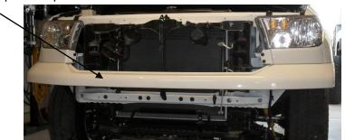
4 Remove aluminum front bumper structure and retain factory hard ware.
