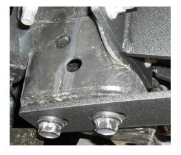
2 Install Front bumper by using the shackle plates by using M 12 hardware. It may be easier to insert one bolt on each side, leaving loose. Then install the remaining 6 bolts. Leave all bolts loose at this time. This will allow for adjustment of the shell to get the fit to the vehicle.
