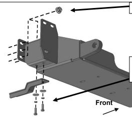
(Fig 13) Reuse factory hex nuts to attach Winch Tray Bracket Assembly to end of frame
