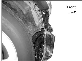
(Fig 6) Plastic cover and facia body panel removed
