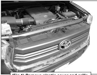
(Fig 1) Remove plastic cover and grille
