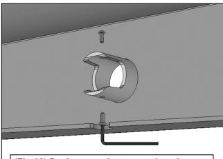
(Fig 18) Push sensor into mounting sleeve. Use 4mm Screws to lock sensor in place.
