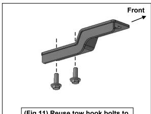
(Fig 11) Reuse tow hook bolts to attach passenger/right Support Bracket to bottom of frame
