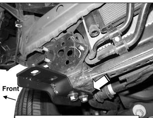
(Fig 12) Reuse tow hook bolts (arrow) to attach passenger/right Support Bracket to bottom of frame
