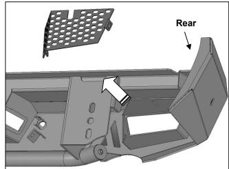
(Fig 12) Remove screens, if necessary, for additional clearance around or access to lights
