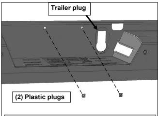
(Fig 11) Push trailer plug into place. Push Plastic Plugs into square holes for license
