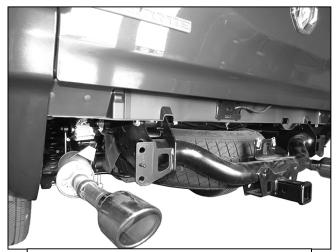
(Fig 4) Factory bumper assembly removed
