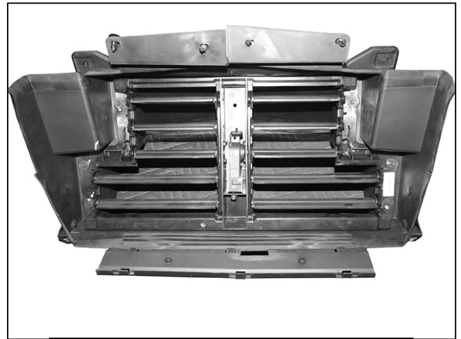
(Fig 2) Unplug shutter mechanism and remove from outer shroud and housing
