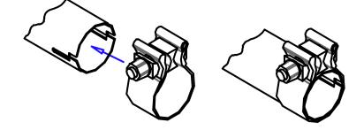
WARNING: Use extreme caution during installation. Torque all fasteners according to manufacturer's torque values and tightening sequence. <u>DO NOT</u> use air impact tools to tighten fasteners on Borla Performance Exhaust Systems. Use of such tools may result in bent flanges or gasket contact areas leading to exhaust leaks.
