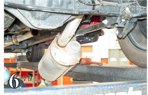
6. Remove the ground clip from muffler assembly hanger.
