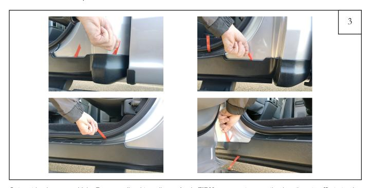
Set part in place on vehicle. Remove all red tape liners. Apply **FIRM** pressure to mounting locations to affix to truck.
