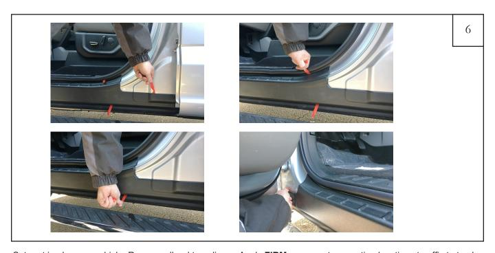
Set part in place on vehicle. Remove all red tape liners. Apply **FIRM** pressure to mounting locations to affix to truck.
