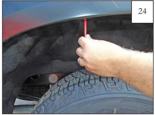
Use a grease pencil to mark the five locations of the holes indicated by the circles in Step 23. Remove flare from vehicle.
