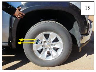
Re-install (2) factory screws (removed in Step 5) with a T15 bit. *Do not tighten*.
