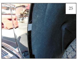
Install supplied Tab (MT1-0034) at each location marked in Step 24.
