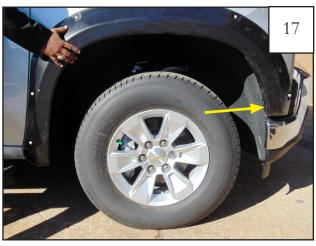
FOR 2019-2022 LTD ONLY: Install (1) supplied phillips head screw (SW1-0049) at front Clip location. *Do not tighten.* (If needed use an awl to align flare mounting holes.)
