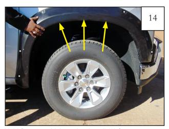
Hold flare to vehicle and re-install (3) factory screws (removed in Step 7) with a T15 bit. *Do not tighten*.
