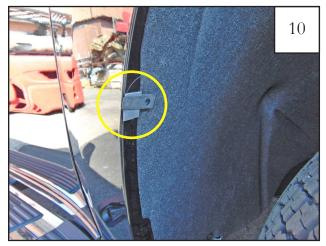
Install supplied Tab (MT1-0034) over the rear location marked in Step 9. Install a Clip (CL1-0009) as indicated on top of the protective film.
