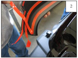
Before placing the part on the vehicle, take the tab for the line of 1/2" tape nearest the lowest curvature of the part and fold it up as shown.
