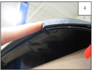
For proper alignment, check that edge of part is hooked over the edge of the hood along entire length of part. NOTE: Hood will not close properly if part is not snug around the lip.
