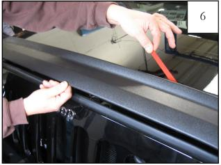
While pulling 1/2" tape liner, move hand to continue pressing on part.
