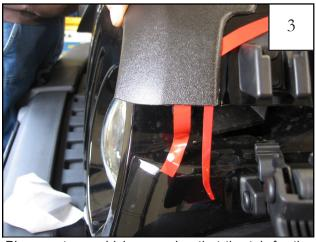
Place part on vehicle, ensuring that the tab for the line of 1/2" tape nearest the front of the hood is positioned as shown.
