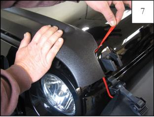
Take the tab of the remaining 1/2" tape strip and pull tape liner. While pulling liner, press on part as was done for first strip of tape liner. NOTE: Take care not to catch tape liner on other piece of tape and accidentally pull its liner off as well.
