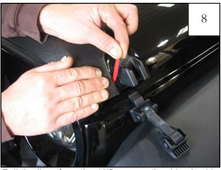
Pull the liner from the 1/4" tape on the driver's side of the vehicle.
