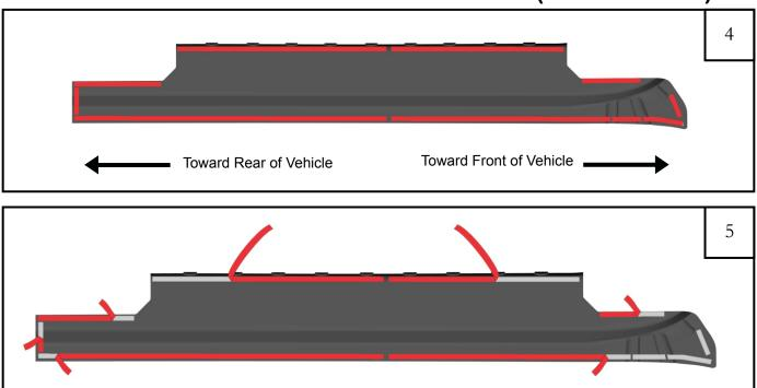
Peel back roughly 3" of red tape liner from the pieces of tape on the back side of the front part. Make sure red tape liner will be accessible when part is attached to truck.
