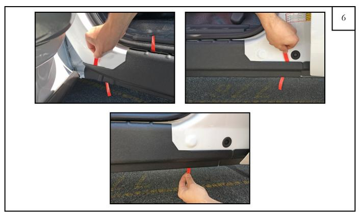
Set part in place on vehicle. Remove all red tape liners. Apply **FIRM** pressure to mounting locations to affix to truck.
