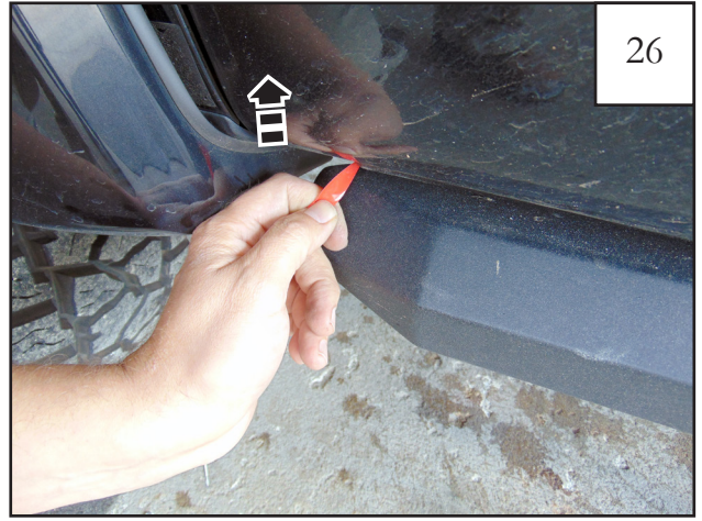
Pull tape liner tab 5. NOTE: It may be necessary to partially close the front door to reach tape tab.
