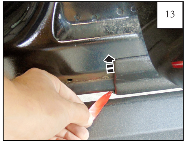
Pull tape liner tab 5. NOTE: It may be necessary to partially close the rear door to reach tape tab.
