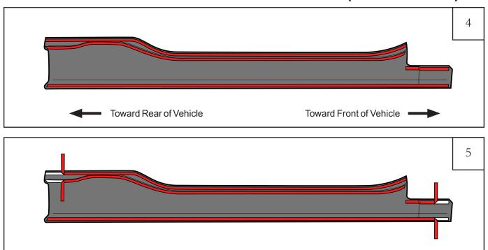
Peel back roughly 3" of red tape liner from the pieces of tape on the back side of rear part. Make sure red tape liner will be accessible when part is attached to truck.
