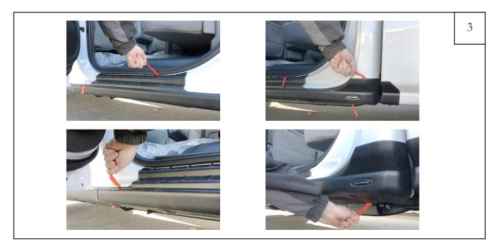
Set part in place on vehicle. Remove all red tape liners. Apply **FIRM** pressure to mounting locations to affix to truck. **NOTE:** Actual application may vary slightly from images.
