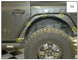
Note (5) locations where rivnuts will be installed in rear fender area.
