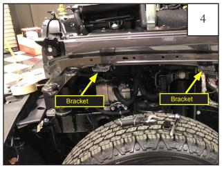
Use a cutting disk to remove the 2 fender support brackets.
