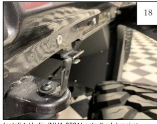
Install 1 U-clip (NU1-0031) onto the L bracket.
