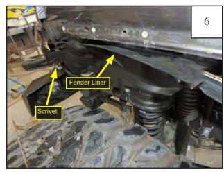
Reinstall the splash shield using the previously removed factory scrivet in preparation for marking before cutting.
