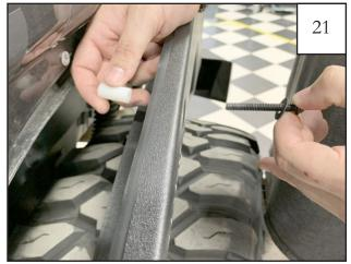
Install front fender delete using 5 bolts (2 short 133606M, and 3 long 1333606G), 5 washers (WA1-0029), and 4 short spacers (SP1-0004).
