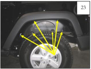
Using a pry tool, pliers, or flat head screwdriver, remove and retain six plastic fasteners from inside of splash shield.
