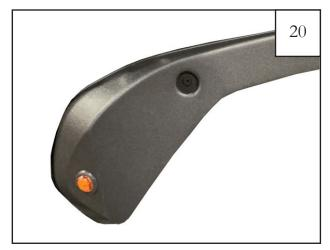
Push round button light through the hole on the front of the fender delete.
