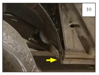
NOTE: It may be necessary to trim the factory installed lower plastic cover piece indicated above to obtain correct fit.
