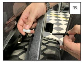
Install rear fender delete using 5 long bolts,(133606G) 5 washers (WA1-0029), and 5 spacers (1 short SP1-0004, and 4 long SP1-0005).
