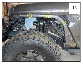
Note (4) locations where rivnuts will be installed in front fender area.
