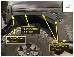
Use the noted hardware combinations to install the fender delete. Install from rear to front loosely. Tighten bolts once all 5 are installed.
