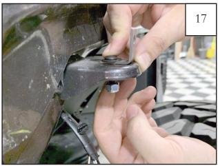
Install L bracket (MB1-0014) on fender support using 1 short bolt (133606M) with 1 washer (WA1-0029) and 1 nut (NU1-00010). Align bracket facing outward and tighten nut.
