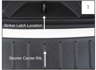
Open rear door of vehicle. WITHOUT peeling liner from tape pads, align part on bumper, the shorter center rib of the bumper protector lining up with the center of the striker latch location.
