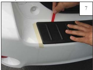
Maintaining part placement, repeat process for final tab liner.
