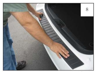
Press the part into place starting at the left side, pushing downward & forward while working to the right. Apply 30 PSI to the taped areas for proper bond. Maximum adhesive bond is reached after 24 hours of contact.
