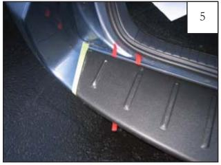
Hold the part at an angle to prevent tape from prematurely sticking and align on the bumper by aligning holes in part with factory holes in bumper and using the masking tape applied in Step 4 as a guide.
