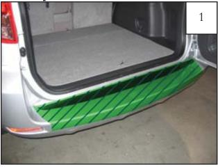
Open rear door of vehicle. Make sure that all installation surfaces are free of dirt and/or grease. Use a clean, lint-free cloth and isopropyl alcohol based cleaner.
