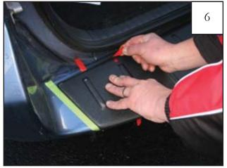
Maintaining part placement, stick peeled end to bumper and begin pulling center tab while applying downward pressure to center tape pad. Repeat for liner nearest the front of the vehicle. Repeat for liner toward the rear of the vehicle.
