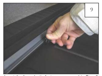
Insert the four plastic fasteners removed in Step 2 through the holes in the bumper protector and into the holes in the bumper threshold. Press into place.
