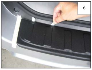
Maintaining part placement, repeat process for center liner with white tab closest to center of vehicle.
