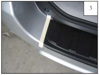
Apply a piece of masking tape along the driver side edge of part for ease of placement during installation.
