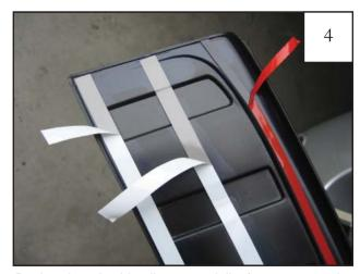
Peel red and white liners partially from tape pads. Center white liner must be peeled back further or it will stick to outer white liner tape pad. NOTE: Make sure tabs are folded toward the outside of the part.
