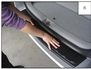
Press the part into place starting at the left side, pushing downward and forward while working your way to the right. Apply 30 PSI to the taped areas for proper bond. Tape reached maximum adhesive bond after 24 hours of contact.
