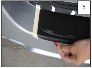
Align the part on bumper by aligning center rib in part with center of striker latch location and using the masking tape applied in Step 3 as a guide. Stick peeled end to Bumper and pull red tab nearest the rear of the vehicle while applying downward/forward pressure to the rear edge of part.
