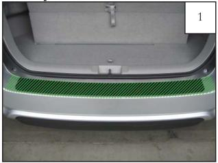
Open rear door of vehicle. Make sure that all installation surfaces are free of dirt and/or grease. Use a clean, lint-free cloth and isopropyl alcohol based cleaner.
