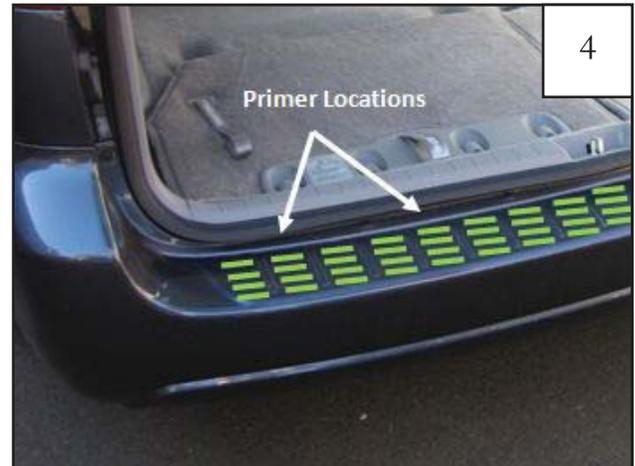
Apply Adhesive Primer to black unpainted part of bumper, between raised surfaces.
