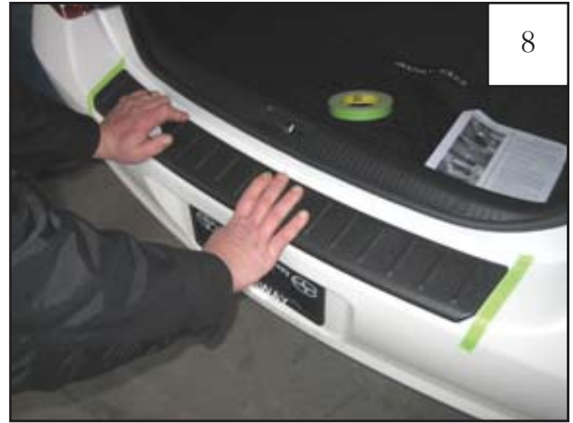
Press the part into place starting at the left side, pushing downward and forward while working your way to the right. Apply 30 PSI to the taped areas for proper bond. Tape reached maximum adhesive bond after 24 hours of contact.
