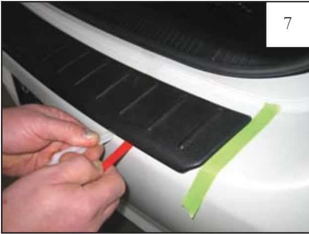
When peeling liner along front edge of part, run edge trim tool along under part in front of liner to create a small gap for ease of liner removal.
