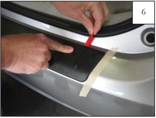
Maintaining part placement, stick peeled end to bumper and pull tab nearest the rear of the vehicle while applying downward pressure to rear edge of part.
