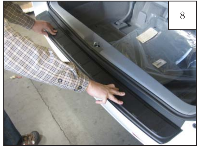
Press the part into place starting at the left side, pushing downward and forward while working your way to the right. Apply 30 PSI to the taped areas for proper bond. Tape reaches maximum adhesive bond after 24 hours of contact.
