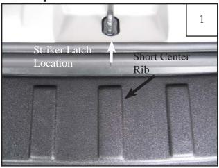
Open rear door of vehicle. WITHOUT peeling liner from tape pads, align part on bumper, centering the center rib of the bumper protector with metal loop on striker.
