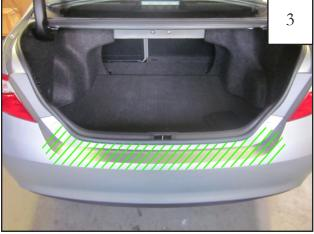
Make sure that all installation surfaces are free of dirt and/or grease. Use a clean, lint-free cloth and supplied isopropyl alcohol-based cleaning pad (AD1-0008).
