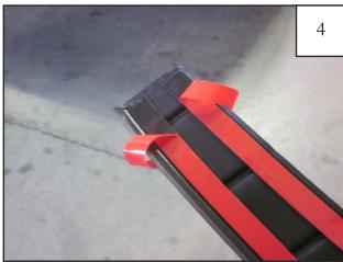
Peel red liners partially from tape pads and fold towards the outside of part.
