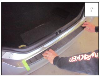
Press the part into place starting at the left side, pushing downward and forward while working your way to the right. Apply 30 PSI to the taped areas for proper bond. Tape reaches maximum adhesive bond after 24 hours of contact. Remove masking tape.
