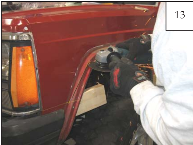
Cut along the horizontal line made in Step 7.
