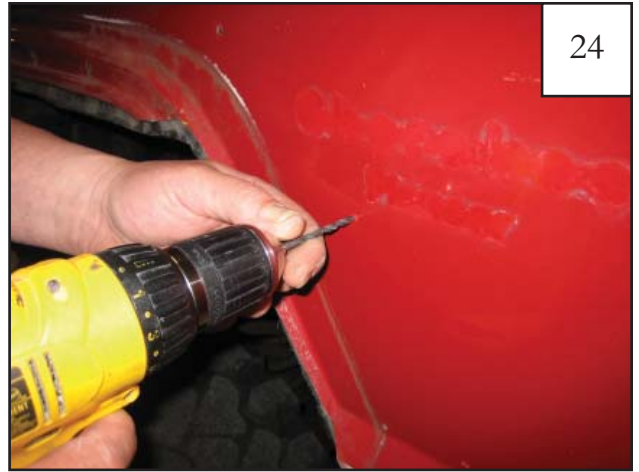
Drill marks with a 3/16" bit.
