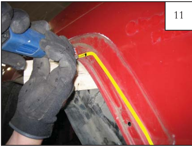
Cut along the horizontal line made in Step 9.
