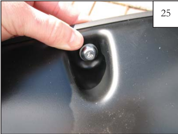
Insert a supplied Torx screw through each pocket in flare.
