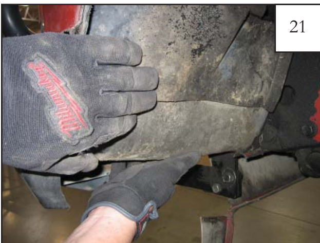
Fold the remaining flap under the bumper.
