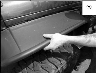
Place the outer flare over the inner pieces and push until snug against the sheet metal. Make sure that the side marker light wires are inside the flare. Make sure splash shield is tucked behind flare.
