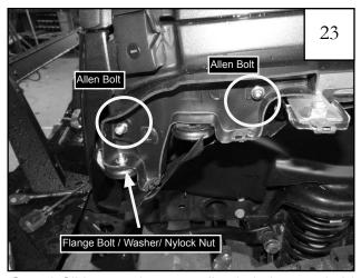
**Step 2** Slide a washer onto allen bolt. Insert a bolt/ washer assembly through inner piece and fender and secure to rivnut. *Start the bolts but do not tighten*. Next, install a 1/4-20 flange bolt and washer with nyloc nut as indicated above. Tighten this bolt fully.
