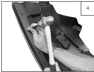
Use a punch or drill with 5/16" bit to drill through eight plastic rivets along edge of flare/splash shield. Discard flare. Save splash shield for reinstallation.
