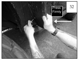
After all screws have been started, tighten the screws by *firmly* pressing the flare toward the vehicle *while* tightening.
