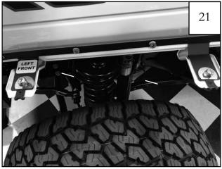
Support bracket flange properly attached to existing factory support in (2) locations.
