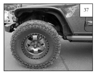
Completed front driver's side flare installation.
