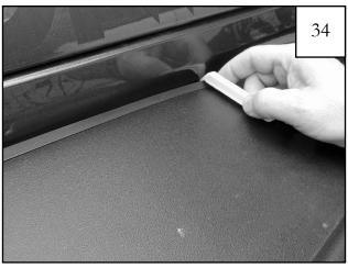
Use the hooked end of the edge trim tool to check for full adhesion. Do this by sliding it along the top of the edge trim to visually verify that the tape is adhered to the vehicle surface. Repeat Step 34 if tape is not fully adhered to the vehicle surface.
