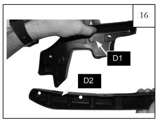
Locate the flat flare front inner pieces. The driver side front inner pieces are marked D1 & D2. The passenger side front inner pieces are marked P1 & P2.
