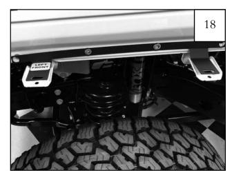
Position support brace along the top edge of fender opening, aligning with the existing factory supports.
