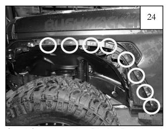
**Step 3** Secure inner piece D2 with allen bolts and washers using the same procedure described in Step 22 and 23.
