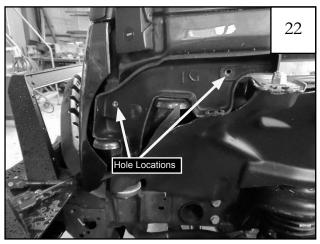
Secure inner piece D1 (and P1 for passenger side installation) to the sheet metal using the following **3 Steps: Step 1** Position inner piece on fender by aligning holes with previously installed rivnuts.
