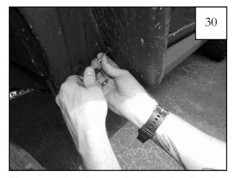
Use a scratch awl (or another pointed tool) to line up the speed clips with the outer flare holes (9 locations). If needed, use a flashlight to better locate the speed clips.
