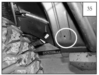
Install a 8-20mm nylon retainer in lower inside corner of fender flare.
