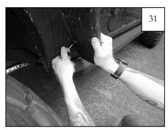
Hold flare in place on fender and start a phillips truss screw into each hole location and through speed clip on inner structure and metal frame angle support bracket (9 locations). Do not tighten.
