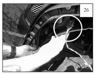
Position inner splash shield for reinstallation, making sure that side marker light wires are outside of splash shield.
