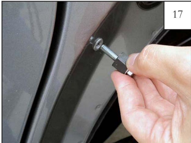
Remove rivnut tool. Repeat for remaining holes.
