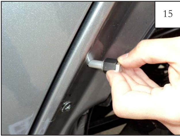
Insert rivnut in fender hole.
