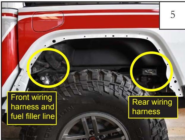
Locate the (2) exposed wiring harness areas inside the rear wheel well. NOTE: The passenger side only has the rear harness.
