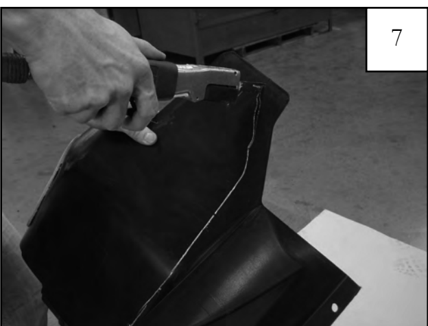
Remove splash shield. Save factory hardware for reinstallation. Using a metal hacksaw, pneumatic hand saw, or other suitable cutting device, trim the splash shield along the marked lines.
