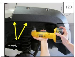
Predrill fender lip at top horizontal area with a 1/8" drill bit through holes in rear main flare (2 places).
