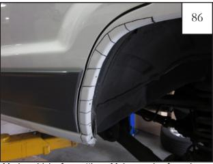
Mark vehicle for cutting: Make marks from inner wheel well to line drawn in previous steps about 2" apart as shown in picture. Make marks closer together around tight corners and style lines.
