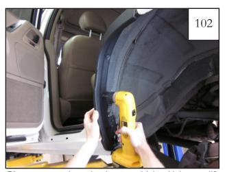
Place cover piece back on vehicle. Using a #2 phillips head, install screws (SW1-0056) through cover piece into holes drilled in step 100. Remove excess caulking along edges if needed.
