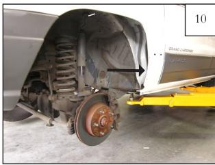
Remove splash shield and push sound dampening foam back into inner wheel well behind the fender. NOTE: If debris is present in inner wheel well, remove before continuing installation.
