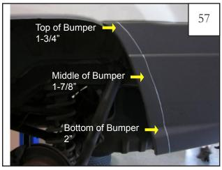
Mark rear bumper for cutting: 1-3/4" at top of bumper, tapering to 1-7/8" in middle of bumper and 2" at bottom of bumper.
