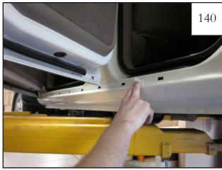
(NOTE: For models with previously removed Rocker Panels) Open front and rear doors. Remove dirt and debris from rocker area around holes in sheet metal. Then use supplied alcohol prep pad to clean and prep area prior to molding installation.
