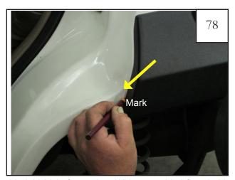
Mark Vehicle for cutting: With assembled flare held in place and aligned with door seam, make a line along front edge of flare.
