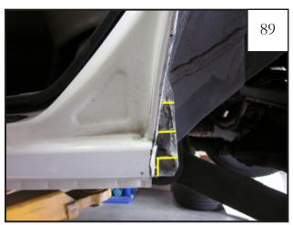
Mark vehicle for cutting: Make horizontal marks on the inner pinch weld flange approximately 1-1/2" apart.
