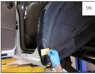
Use a spreader to smooth and evenly spread caulking along cut areas. Allow caulking or primer to partly dry before proceeding. Does not need to be fully cured.
