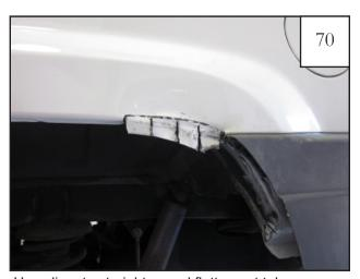
Use pliers to straighten and flatten out tabs.
