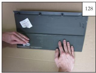
In preparation for applying new tape, use a supplied alcohol wipe (AD1-0010) to clean plastic and remove factory tape from side cladding.
