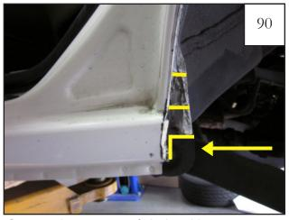
Cut away lower corner of pinch weld.
