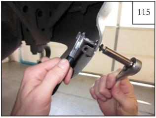
Using a Phillips screwdriver and a 3/8" socket wrench, tighten the nut and screw together.
