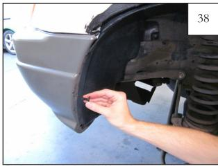
Re-install splash shield using supplied panel retainers (RV1-P008). See next step for retainer locations.
