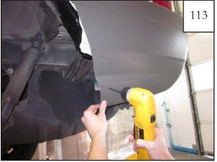
Using a 3/16" drill bit, drill the two holes marked in step 112.
