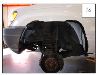
Completed cut-out with caulking applied.
