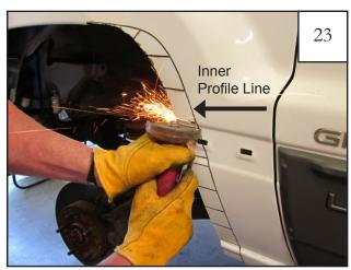
Using a cut off wheel or other suitable tool, cut along horizontal marks from wheel well to inner cut profile line.
