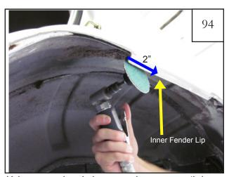
Using an angle grinder or sandpaper, smooth inner edge of fender lip 2" back from edge of cut.
