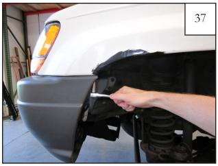
Using a 10mm socket & wrench, re-install factory screw attaching bumper to fender.
