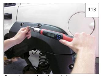
Once all screws have been started, snug screws to vehicle. Torque to 24 in•lb (2 ft•lb). DO NOT OVERTIGHTEN!
