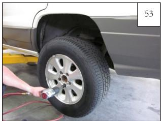
Remove tire using an impact wrench.
