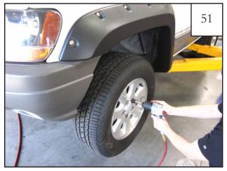
Re-install tire using an impact wrench.
