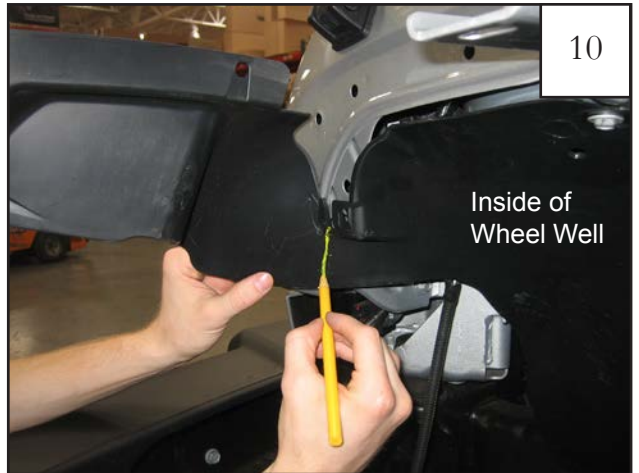
Mark the front portion of the splash shield with a grease pencil in location shown. The splash shield should be flush with the sheet metal after being trimmed. NOTE: If trimmed too little, flare won't fit; if trimmed to much, shield won't stay behind flare.
