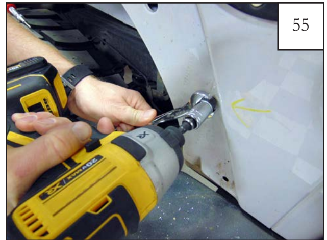
Install rivnuts in locations drilled in Step 54 , using rivnut installation tool.
