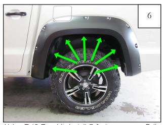
Using T-45 Torx bit, install 7 factory screws. Fully tighten all screws while pressing in on flare to ensure it is snug against sheet metal.
