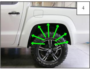
Using an T-25 Torx bit, remove 7 factory screws. Retain screws for reinstallation.
