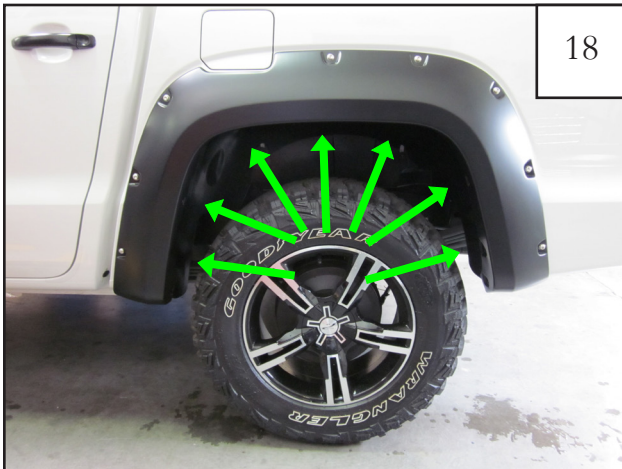
Using T-25 Torx bit, install 7 factory screws. Fully tighten all screws while pressing in on flare to ensure it is snug against sheet metal.
