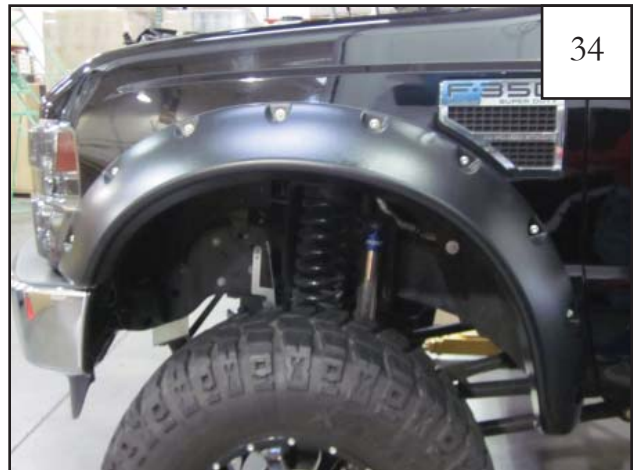
Completed front flare installation.
