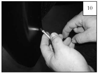
Install four supplied Screws (SW1-0050) through remaining holes and into clips installed in Step 8, working from front to back of wheel well.
