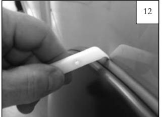
Using supplied Edge Trim Tool (ET1-0002), seat edge trim against vehicle by hooking curved end under edge trim at one end of flare. Next, slide around outer edge of flare to the other end.
