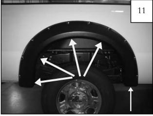
Ensuring proper flare placement, tighten all screws.
