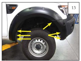
While holding Front Flare/Bumper Peice Combo on Vehicle start six (6) supplied Screws (SW1-0056) into flare and into clips installed in steps 10 & 11.
