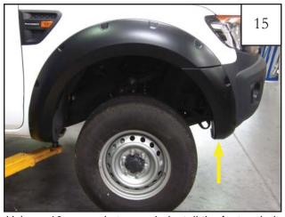
Using a 10mm socket wrench, install the factory bolt that was removed in step 8 under the front bumper area of wheel well.
