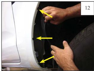
Peel back the rear wheel well liner and install three (3) supplied clips (CL1-0022) at the three locations indicated. Replace liner to original position.
