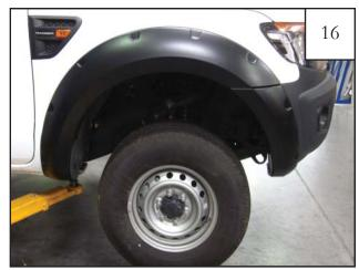
Tighten all screws. Front flare installation complete.
