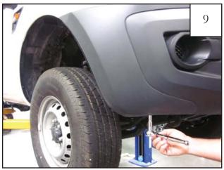
Using a 10mm socket remove One (1) factory bolt from under front bumper area of wheel well. Save factory bolt for reinstallation.
