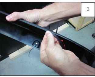
Press edge trim into place along the top edge of the flare in one-foot increments, pulling red vinyl backing free as you continue to work your way around the top edge of the flare.
