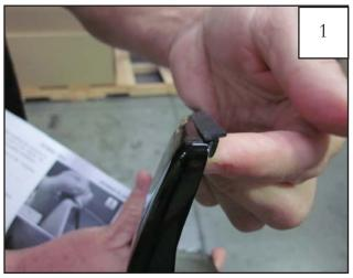
Peel two to three inches of red vinyl backing away from Edge Trim (GP1-0007) tape. Applying the adhesive side of the edge trim to the inner side of the flare, affix the edge trim to the top edge of the flare (the portion that comes in contact with the vehicle).
