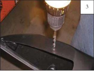
(Optional) Using a 5/16" bit, drill holes at indents located at the ends of Front Main and Front Bumper Pieces. Two places each part.
