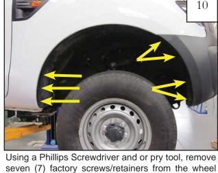
Using a Phillips Screwdriver and or pry tool, remove seven (7) factory screws/retainers from the wheel well and discard. *Note:* Some vehicle models will have factory mudflaps. These will need to be removed for proper installation of flares.
