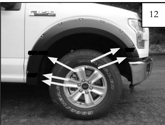
Still holding flare to fender, re-install remaining factory screws removed in Step 4 using 7/32" and 9/32" sockets and wrench. Using a phillips screwdriver, install supplied screw (SW1-0058) into Clip (CL1-0009). Tighten all screws.
