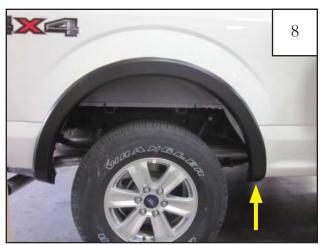
Start a supplied screw (SW1-0050) through the flare into the clip installed in Step 6. Tighten all screws.
