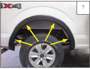
While holding flare to vehicle, start supplied screws (SW1-0058) through the four topmost mounting holes in flare and into the clips installed in Step 5.
