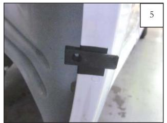
Install a Clip (CL1-0009) over each of the four Tabs (MT1-0034) placed over the upper 4 marks made in Step 3.
