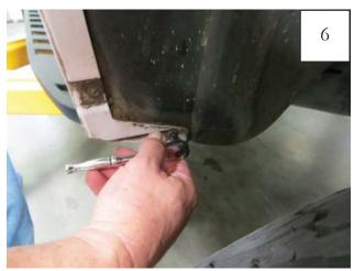
After removing factory flare, use a 7/32 socket to remove the factory screw located at the bottom rear of the wheel well. Retain screw for re-installation.
