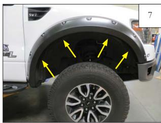
Position flare on fender and install supplied push retainers (RV1-P001) through holes in flare and into factory holes. (4 places)
