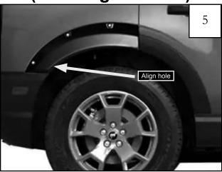
Position rear piece of flare on vehicle. Align the hole in the back of the flare with the factory hole.
