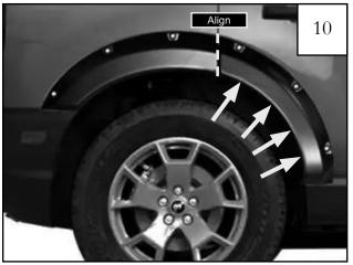
Position and align the remaining portion of rear flare on vehicle. Note the (4) slotted fastener locations in the flare. Repeat **Steps 8-10.** Check door function and adjust placement of flare as needed.
