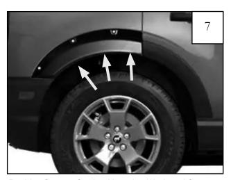
Position flare on fender. Note the (3) slotted fastener locations in the flare.
