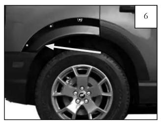
Install one fastener (RV1-P006) in the rear hole.
