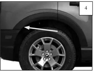
Remove (1) factory installed plastic fastener from the rear of the wheel opening to expose hole.
