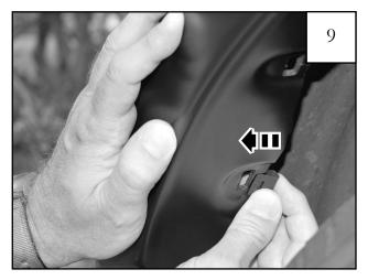
Press U-clip (122411) in place so that it encompasses both edge of fender flare and edge of factory fender trim, making sure that the retension tang of the U-Clip engages in the slot. Repeat for remaining slots.
