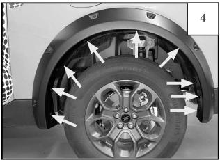
Hold rear flare up to vehicle wheel opening. Use a grease pencil to mark (9) locations where factory fasteners will need to be removed from the wheel opening.
