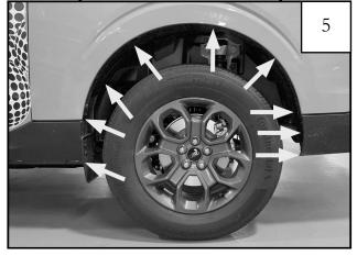
Set fender flare aside. Remove (9) factory fasteners from marked locations. Retain fasteners for reinstallation.
