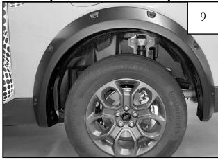
Completed rear fender flare installation.
