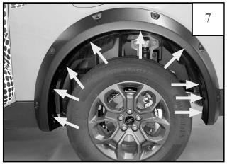
Position fender flare back in place on wheel opening and align with holes. Reinstall (9) previously removed factory fasteners and screws.
