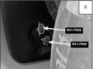
Install (1) RV1-P006 fastener and (1) RV1-P008 fastener in the remaining (2) holes where the mudflap was originally installed. (See Frame 6)
