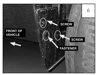
Remove (2) screws and (1) fastener from mud flap in front of rear tire. Screws, fasteners, and mudflap may be discarded.
