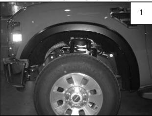
Using a 7/32" socket, remove four factory screws. Retain screws for later use.
