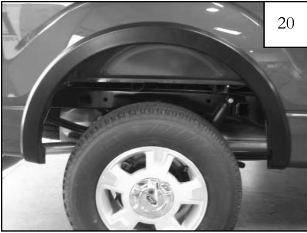
Completed rear flare installation.
