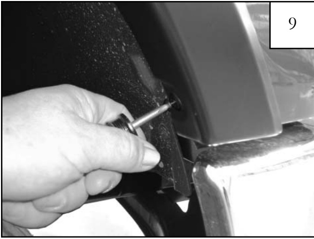
Still holding flare to fender, install tuflocks using a Phillips screw driver. See step 10.
