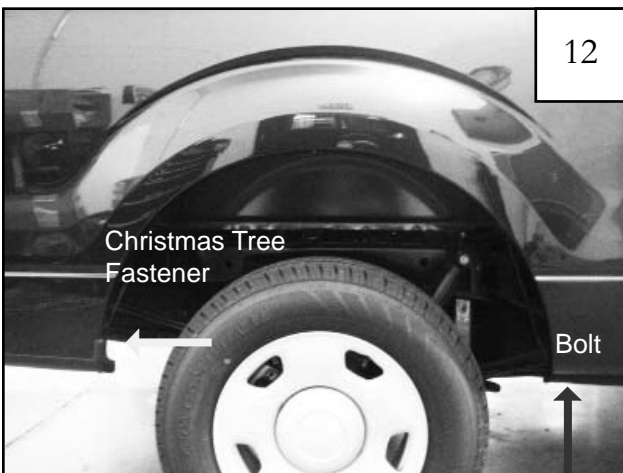
Remove one factory bolt from the forward, underside of the rear wheel well with a 10 mm socket wrench. Remove one Christmas tree fastener from the inside of the rearward inside of the rear wheel well with a trim tool.
