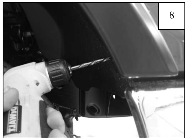
Still holding flare in position on fender, drill through bumper cover with a 1/4" drill bit using the forward most hole in the flare as a guide.
