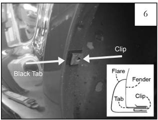
Install a clip over each of the black tabs installed in Step 5.
