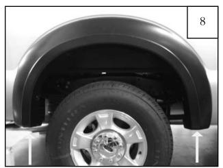
Using a 5/32" Allen Wrench and 3/8" Socket, install bolt, silver washer, spacer, fender washer, and nut through bottom two holes in flare and into factory holes. See step 9.
