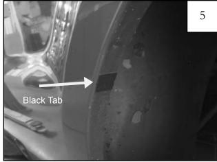
Install a black tab centered over each of the four holes noted in Step 4, and wrapped around the metal lin
