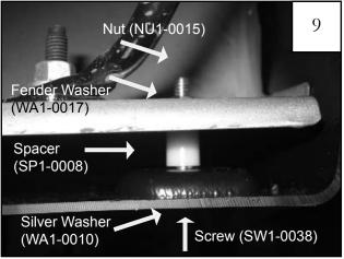
Start bolt (SW1-0038) from the bottom through a silver washer (WA1-0010) and into flare. Install spacer (SP1-0008) between flare and sheet metal. Slide a fender washer (SW1-0017), then the nut (NU1-0015), over the end of the screw.
