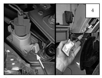
Squeeze the lower tab on the back of the side marker light assembly and remove from the truck. Carefully turn the wiring harness counter-clockwise and separate the bulb/wiring harness from the side marker light assembly.
