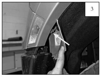
Pull back the fender liner near the front of the fender and locate the side marker light assembly and wiring.
