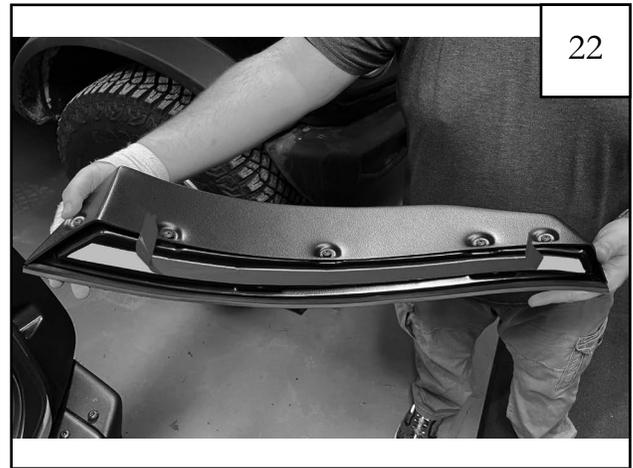
Peel back 2" (5 cm) of tape liner from rear door inner bracket.
