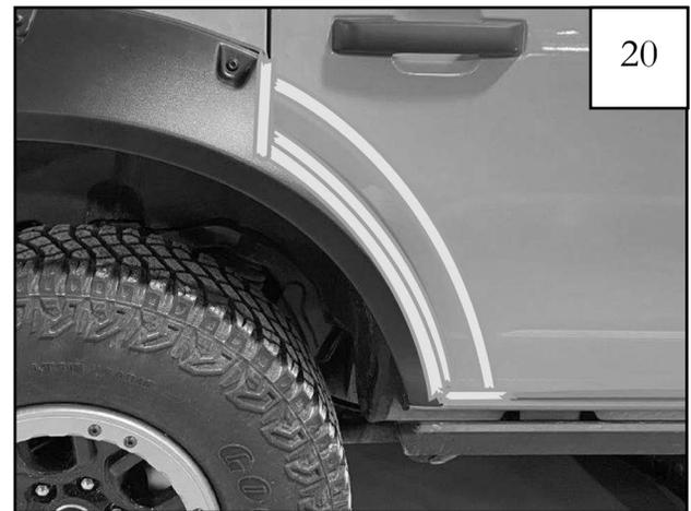
Mask off the areas surrounding where the red tape liner on back of the rear door inner bracket will contact the door surface.
