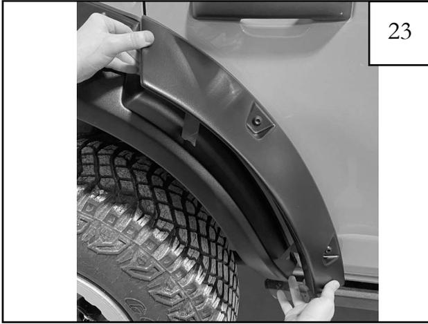
Line up rear door flare assembly to door and main rear flare piece. Ensure clearance to main rear flare in order to open and close door properly. Tack door flare assembly in place.
