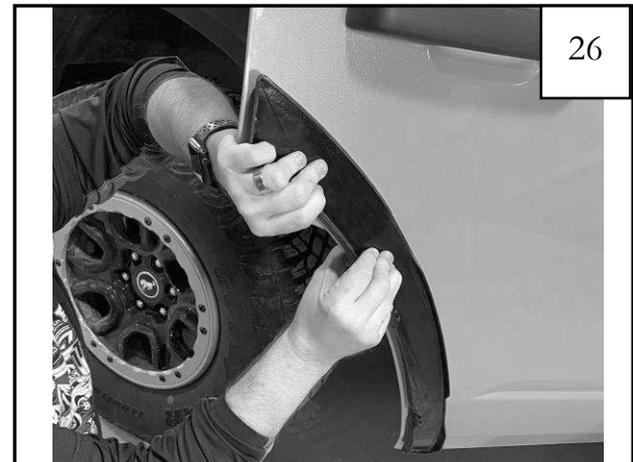
Apply firm pressure to rear door inner bracket to ensure adhesion to surface.
