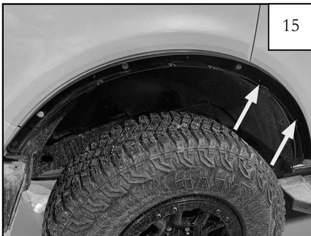
Use (2) SW1-0008 bolts, (4) WA1-0015 washers, and (2) NU1-0016 nuts to complete bracket installation.
