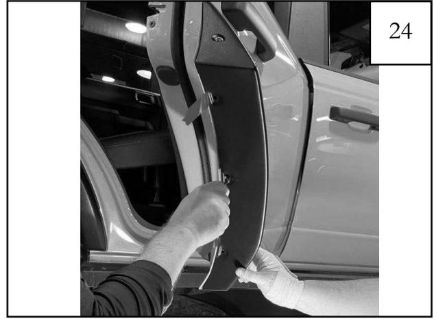
Open door and temporarily remove the previously installed (5) SW1-0058 screws in order to separate the rear door flare from the rear door inner bracket.
