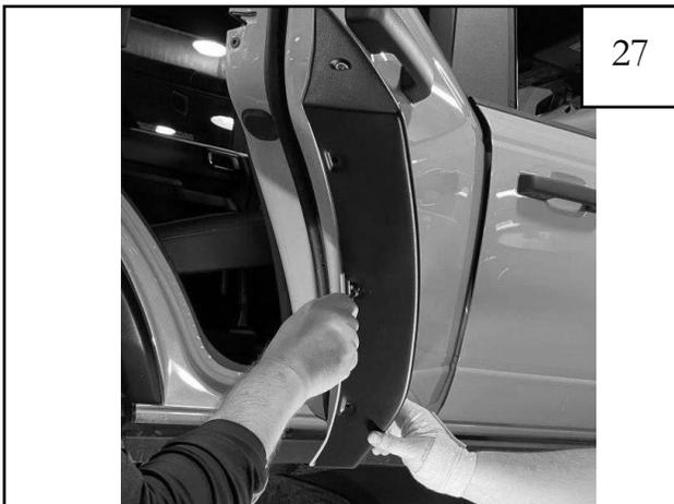
Reinstall (5) SW1-0058 screws to reattach the rear door flare to the rear door inner bracket. **NOTE:** Ensure that edge trim is seated correctly.
