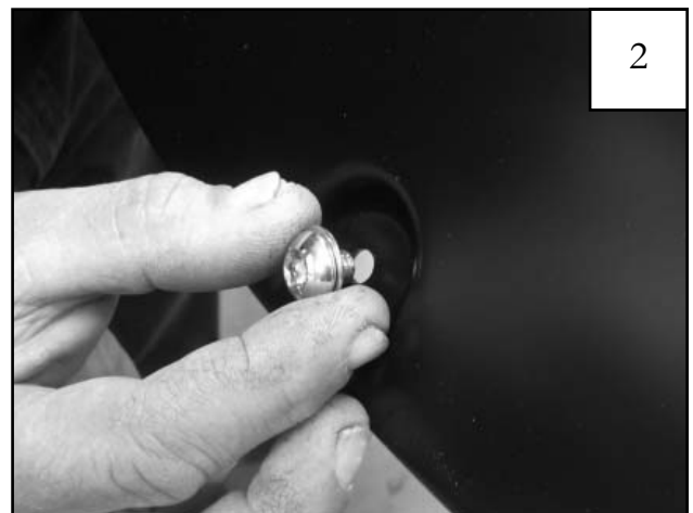
FRONT MAIN & REAR FLARE ONLY: Put each Bolt/Washer combination through a pocket hole in the flare, Bolt head and Washer on the outside.
