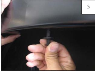
Holding flare in position on fender, install two Plastic Push Retainers in locations shown in Step 4.
