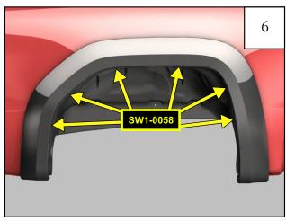
Install rear flare using (6) SW1-0058 truss screws and the (2) outboard screws removed in **Step 1**.
