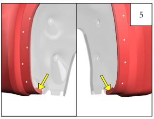
Tuck the fender liner behind the sheet metal flanges at the bottom of the fender. (Plastic fender trim hidden for clarity)
