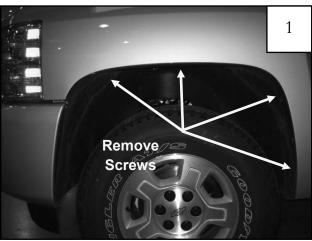
Using a 7mm socket, remove four factory screws. Keep screws for later use.
