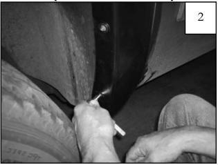
Position flare on fender, and reinstall four factory screws removed in Step 1. If needed, use an awl to locate holes. Note: Make sure flare slides OVER plastic fastener located inside wheel well. If it catches on fastener, it will not fit properly.
