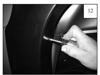
Start a supplied Serrated Flange Screw through each of the remaining holes and into each "S" Clip installed in Step 10. If needed, use awl to locate holes. *Note: It is helpful to install the two bottom screws first.*
