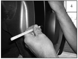
Holding flare in position on fender, use a grease pencil to mark six hole locations. *Note: Rear flares look similar. Verify that you have the correct side prior to installation.*
