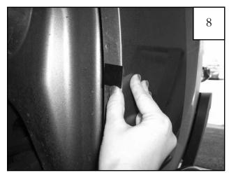
Center a supplied Black Plastic Tab over the six marks made in Step 5, aligning edge of tab with inside of fender lip (tab may extend over outside of fender).
