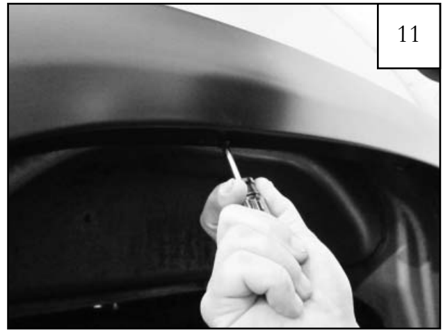
Reposition flare on fender, Start a supplied Screw (SW1-0058) through the two uppermost holes in the flare and into each Clip installed in Step 7.
